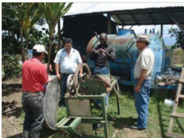
FIGURE 11.9: The TUSIP Research Assistant Checking a Simple Fodder Chopper in Santa Cruz de Turrialba (Costa Rica)
