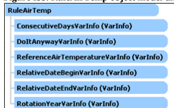
Figure I35. RuleAirTemp object model diagram showing the parameters needed by this rule
