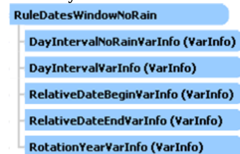
Figure I38. RuleDatesWindowNoRain object model diagram showing the parameters needed by this rule
